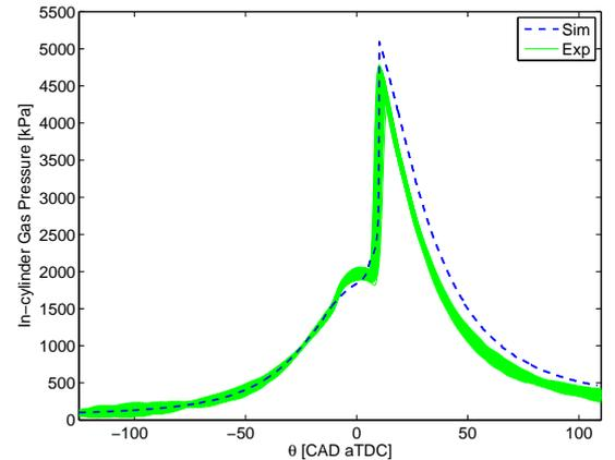
Figure 1: Comparing simulated and experimental pressure traces for test point #14 in Table 2.
